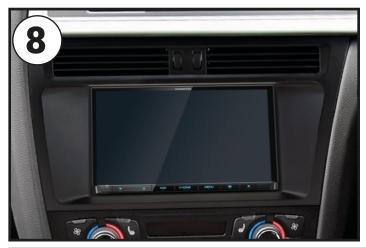
After connecting all the necessary wiring, begin to install the new Double DIN Fascia with the aftermarket head unit into the dashboard.
