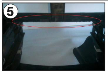
Using a blade or dremel tool, proceed to cut the portion of the interior dash highlighted. This allow the new head unit to sit higher and in align with the fascia plate.
