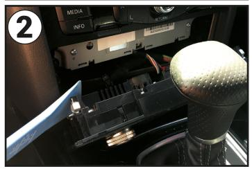
Using the Bojo tool again, pry away and unclip the bottom HVAC panel.
