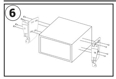
Attach the new Double DIN Brackets to the aftermarket head unit utilising the screws within the kit.
