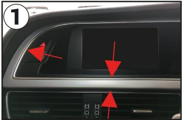
Begin by using a Bojo tool (or similar variant) to pry away and unclip the trim that surrounds the top screen. Once loose, disconnect the hazard switch connector and place to one side.
