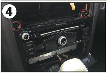
Unscrew the two bolts that hold the head unit into place, when free, remove the head unit and disconnect all the wiring.
