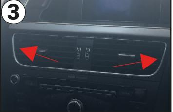
Using a pick tool, insert it in between the fan blades and release the spring clips.
