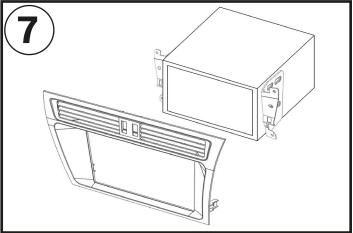
With the brackets attached to the head unit, offer the whole unit to the back of the new Double DIN Fascia. Use the plastic inserts at the bottom of both the Brackets and the Fascia as a guide.
